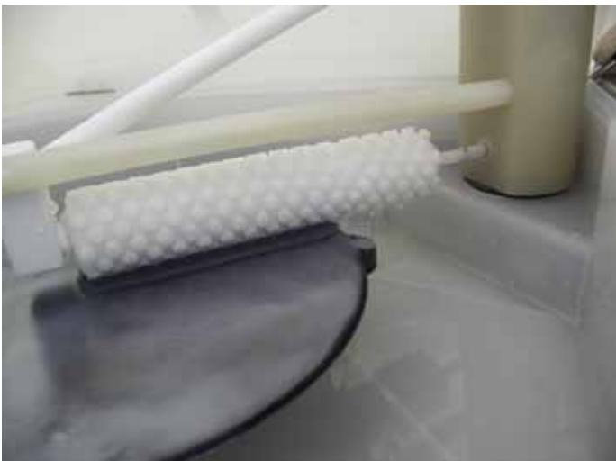
CMP Wafer Cleaning with Brush
