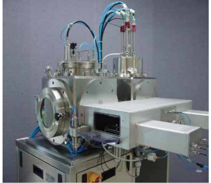
Load Lock and Automatic Transfer Between Chambers w/o Exposure to Atmosphere
