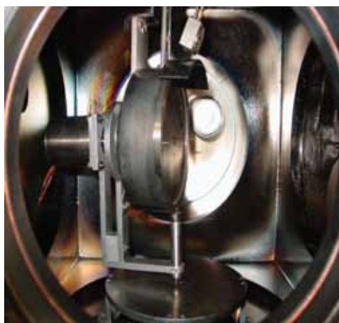
Combinatorial Sputtering System: Dual Side Sputter Housing/Vertical Platen 600 °C Rotating Platen with Tilt and Masking
