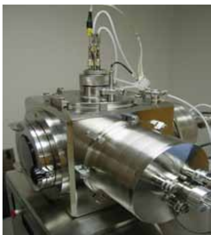
Combinatorial Sputtering System: Dual Side Sputter Housing/Vertical Platen 600 °C Rotating Platen with Tilt and Masking
