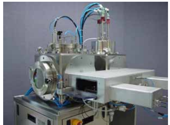
Load Lock and Automatic Transfer Between Chambers w/o Exposure to Atmosphere
