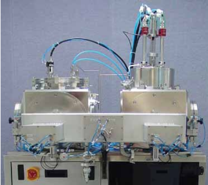
Load Lock and Automatic Transfer Between Chambers w/o Exposure to Atmosphere
