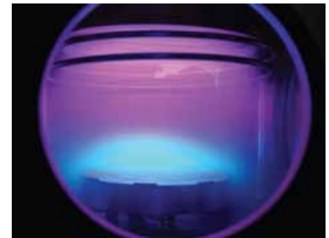
-1000 V DC Bias, 500 °C, ICP On
