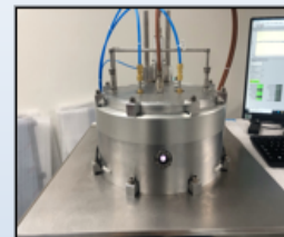
Fig 5. PAALD/PECVD Plasma ON
